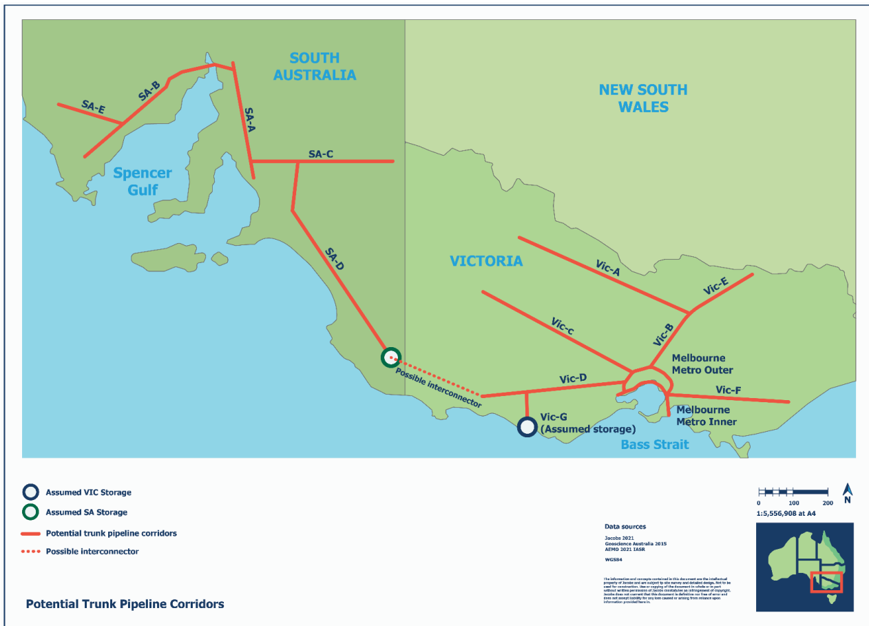
Figure 17: Hydrogen transmission network concept (with possible long-term storage sites)
