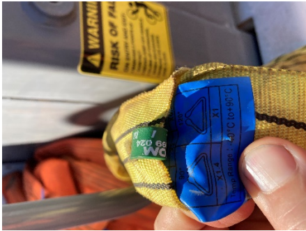
Green tag on Welding Marooka – out of date
